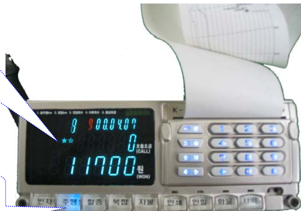
Photo #3: VFD Indication Section & Current Mode Indication with Back-Light
